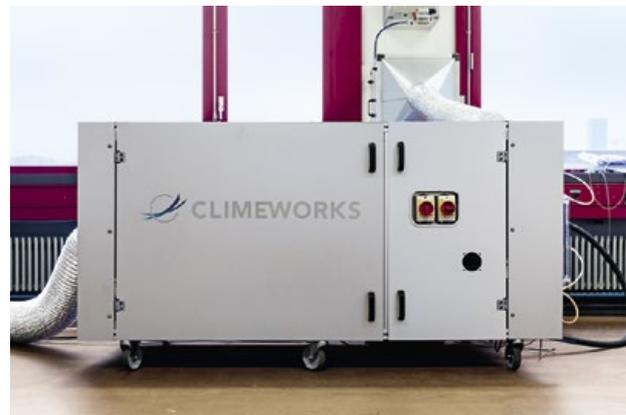
Up to four kilos of CO<sub>2</sub> can be filtered from the air each day: Climeworks demonstrator.
