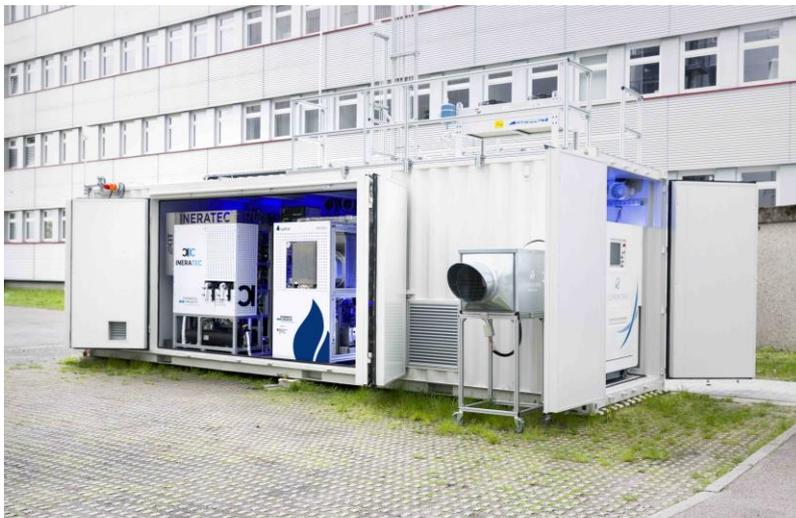
*The world's first integrated Power-to-Liquid (PtL) test facility to synthesize fuels from air-captured carbon dioxide. (Photo: P2X project/Patrick Langer, KIT)*
